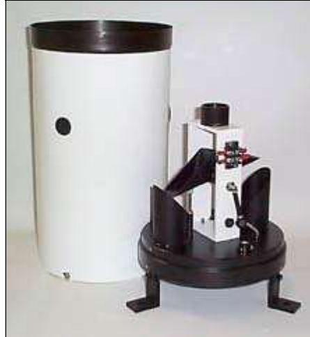
Exhibit 3-3. Tipping Bucket Rain Gage ( http://www.arm.gov/instruments/instrument.php?id=rain )
